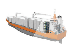
Carbon Capture Retrofit
